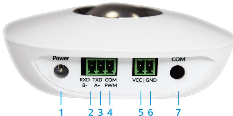
1. DC jack specifications (5.5 mm x 2.5 mm), please use a DC plug 5.5 mm x 2.5 mm. Vcc = 7 – 24 V
