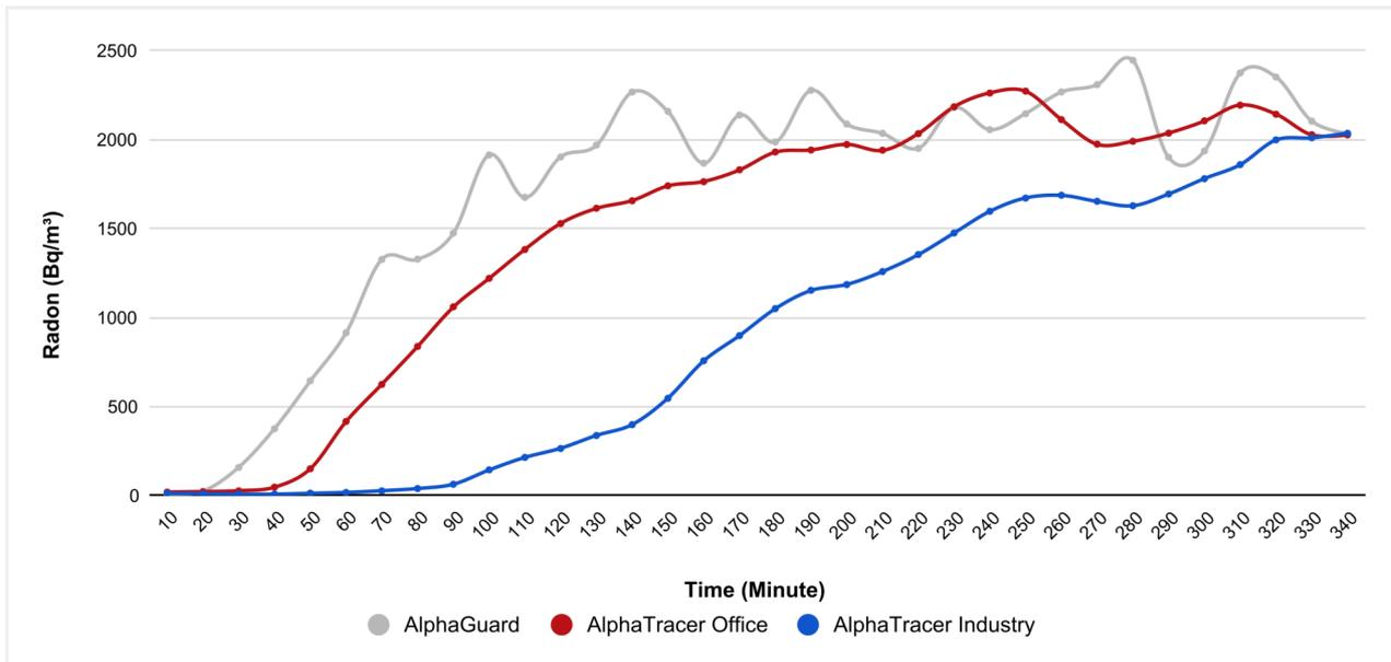
In this example, we have induced (under laboratory conditions) a very rapid increase in the Radon-222 activity concentration from 30 to over 2,500 Bq/m<sup>3</sup>:
