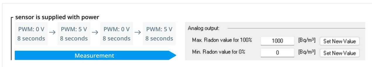
Graphical visualization of the test signal
