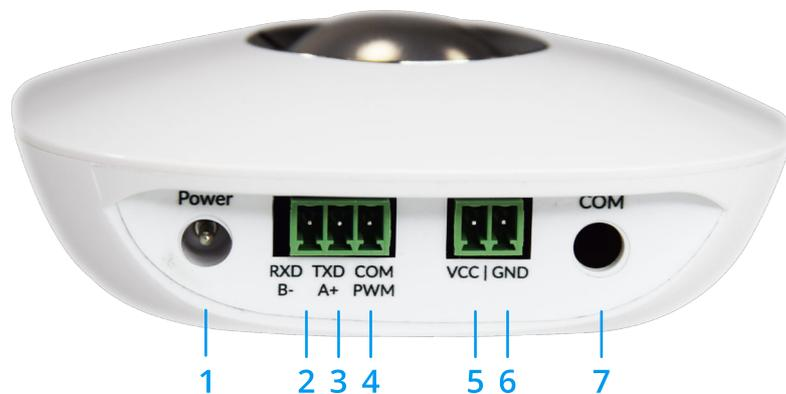
1. DC jack specifications (5.5 mm x 2.5 mm), please use a DC plug 5.5 mm x 2.5 mm. Vcc = 5 V
