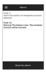
Alarms and warnings are displayed in this menu. Alarms are marked in red, warnings are marked in black. Alarmindicates a serious error in operation. The ventilation system is forcibly switched off.
