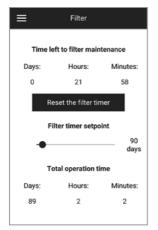
Filter timer setting: After the set time (70-365 days), the filter change indicator appears and the corresponding filter change information is displayed in the alarm menu.
